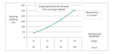
Stopping Distance for Derailed Train running on Ballast
