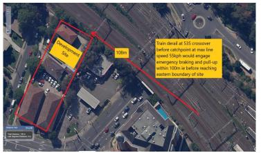
Most unlikely derailment scenario (ref 6 Map diagram above): Train derails at max line speed 55kph ie 30kph above boarded crossover speed, before reaching catchpoint and travels toward Homebush:
